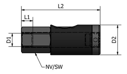
D1 = G 3/8 D2 (mm) = 26 L1 (mm) = 10 L2 (mm) = 75.5 SW (mm) = 21 Weight (g) = 121
